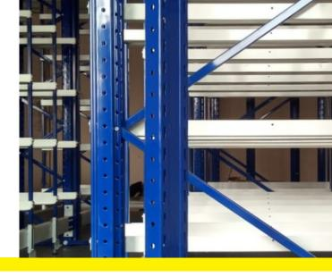
The frame legs are made of special cold-rolled steel profiles. The spacers and braces are made of metal profiles and are bolted to the frame uprights. The frame legs are supported by the thrust bearings. The footrests are fixed to the floor using anchor bolts.
