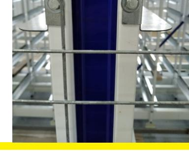
A metal mesh (Gitter, 3D) PPK 50\*200mm (4P) d4 2\*2.5m is used as a protective fencing of the shelving.
