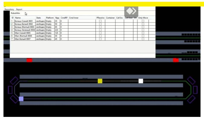
The control system PC is located anywhere in the warehouse at the request of the customer. It is a monitor with a diagonal of 23.6". With a touch screen, at the request of the Customer. All AS/RS processes are displayed on the monitor. The position of all containers, robots, conveyors is displayed, stored and can be retrieved from the system at any time, including in the event of an emergency shutdown.
