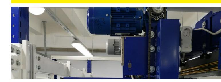
Locomotive provides movement of the robot-stacker along the upper guide rail in the horizontal and vertical direction along the racks. The drive wheels are shrink-fit on the axle, which makes this design one-piece. This method ensures the reliability and integrity of the assembly even under heavy loads and stretching of the metal with alternating motion.
