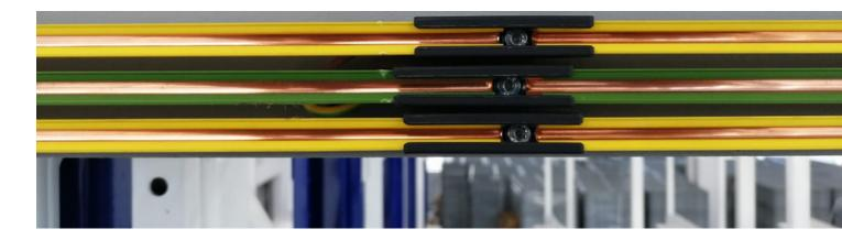
The stacker robot is powered via a bus bar that is attached to the top guide rail.
