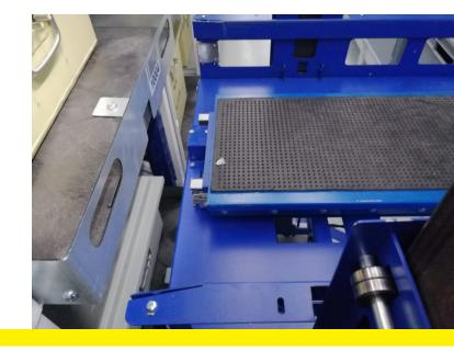
Picks up the container from the rack and also places the container on the rack. The extractor serves containers that are located on both sides of him.
